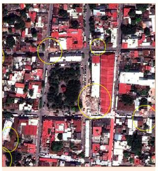
Figure 4: Drone image over Juchitan, Oaxaca, showing collapsed buildings after the 8.1 magnitude earthquake on 7 September 2017.
