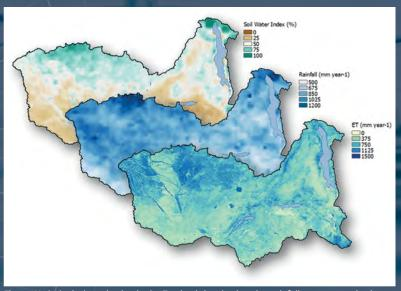
Figure: Hydrological monitoring in the Zambezi river basin using rainfall, evapotranspiration and soil moisture information from multi-source satellite observations.
