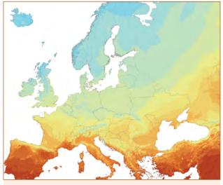
**Figure 3**: Map of photovoltaic solar electricity potential based on Meteosat solar irradiance climatology *Source: JRC with inputs from CM SAF*
